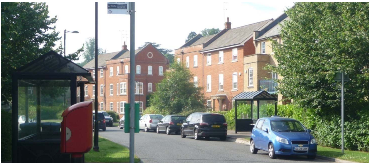
Fig 29: Illegal and inconsiderate parking makes it impossible for bus stops to be used safely. Parking bays or a stop buildout would have been appropriate in this street
