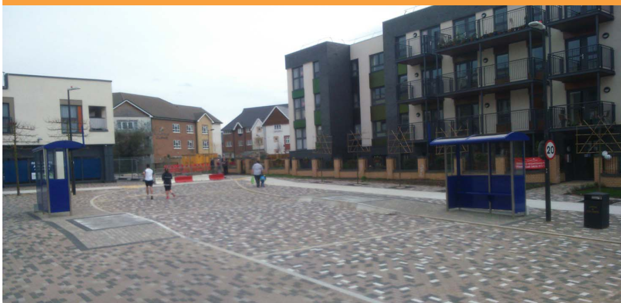
Fig. 11: This pair of stops in a shared space local square presents significant hazards. A stopped bus is likely to block the vehicular carriageway entirely. Note the treatment of boarders and the road surface, which does delineate the vehicular carriageway.
