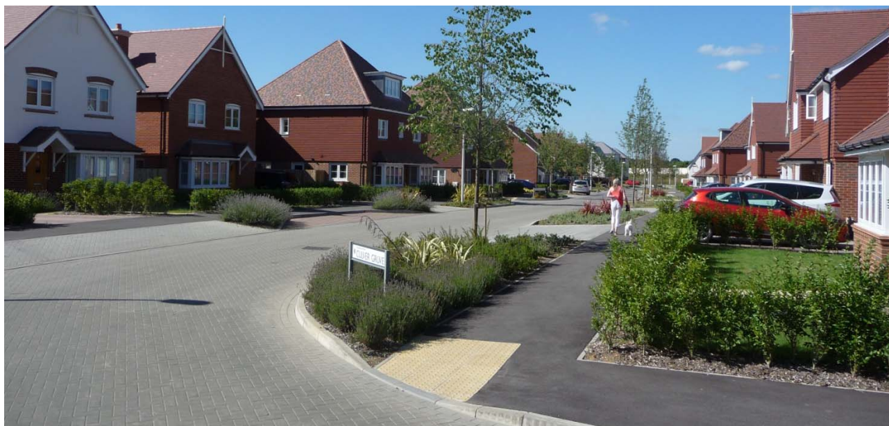
Fig.39 : Wokingham Northern Extension. This primary street achieves an excellent balance between multiple urban design requirements. Parking in front of plots, and lavish planting, can co-exist while keeping a carriageway largely free of parking..
