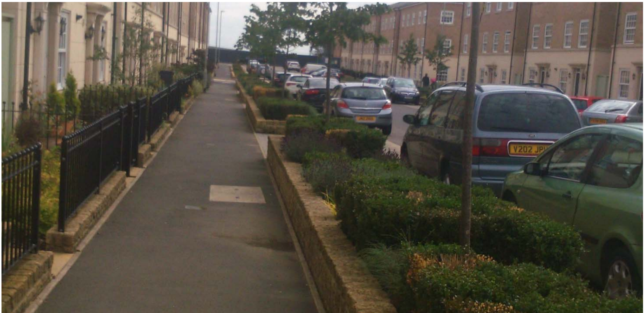
Fig 7: Corby Priors Hall: parallel parking bays are provided continuously off-street. Planters add a further buffer between the main street carriageway and both pedestrians and habitable rooms, in a high-density development featuring continuous frontages.
