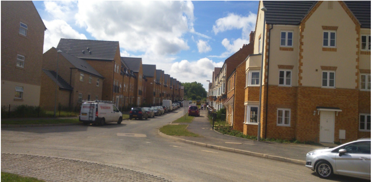
Fig. 40: This length of primary street, and two stretches either side out of view, are reduced to single carriageway for over 500m. Note too, inappropriate parking on the verge; and on the circulatory carriageway of a roundabout.
